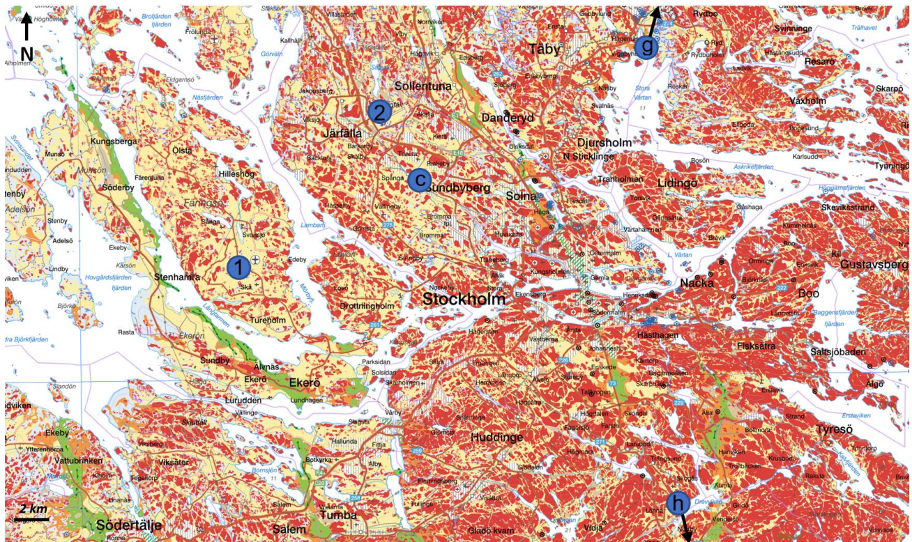
Figure 2. Geological map over western part of Stockholm. Areas in yellow are clay (both glacial and post glacial deposits), areas in red are near-surface bedrock and areas in green is till or esker (adapted from [19]). Point with letter refers to photographs in Figure 4. Point marked with “1” denotes the location of the Skå-Edeby test field set up by SGI in 1957, and point “2” refers to location of mini block sampling presented herein.
