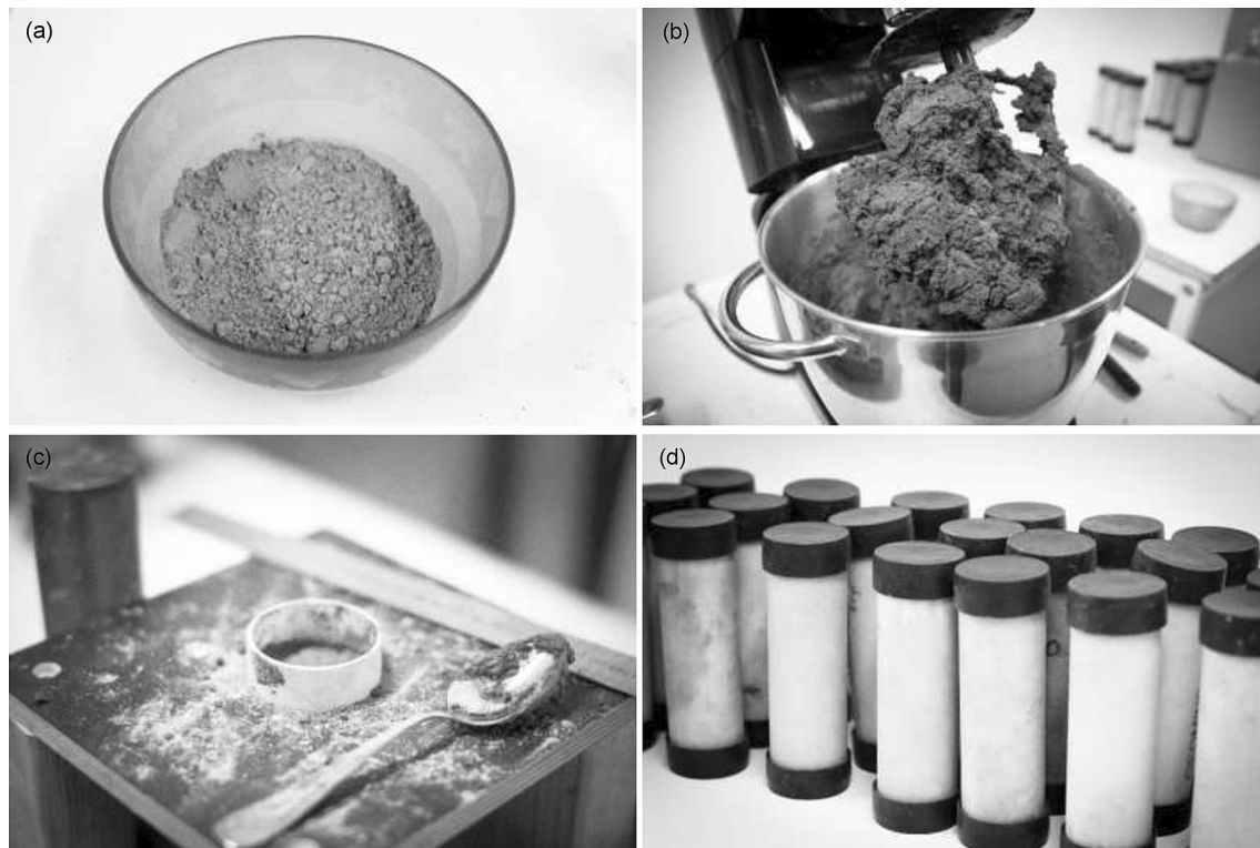
Fig. 2 Specimen preparation, a pre-mixed dry binder, b homogenising of mixture, c moulding in reinforced plastic cylinders, d sealed cylinders under curing
